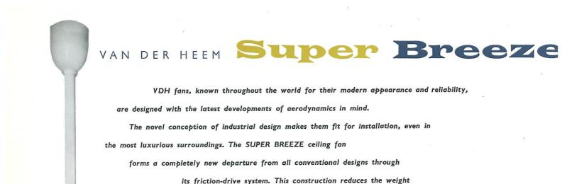
The reliable condensormotor has an extraordinary low power consumption and produces a large air displacement. Special metal alloys and multiple lacquering stand up to the most torrid climates. The double insulated, rubbercushioned suspension cuts down noise
